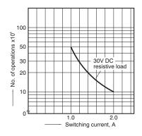
3. Mechanical life Tested sample: TX2-5V, 10 pcs. Operating speed: 180 cpm
